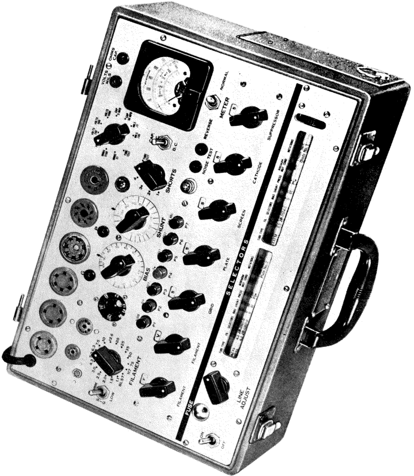
Figure 1-1. Tube Tester TV-3/U with Cover Removed
