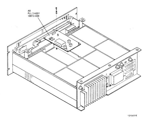
Figure 1. PLL 3 Assembly A8 Location
