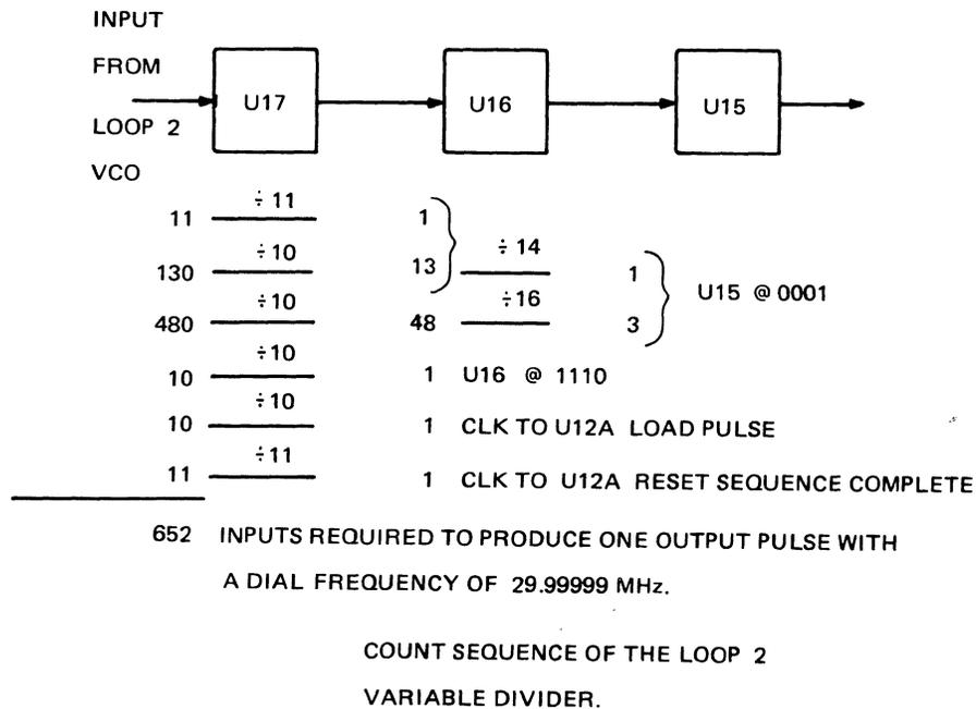
Figure 5-4. Count Sequence of the Loop 2 Variable Divider.
