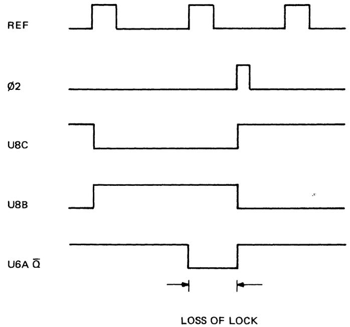
Figure 5-10. Variable Reference Frequency Loop Frequency-Phase Detector Waveforms.
