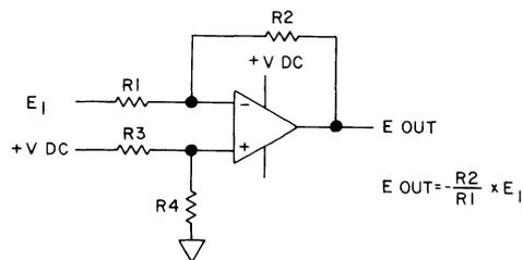
Figure 9-13.3. Inverting Amplifier with Offset Voltage.
