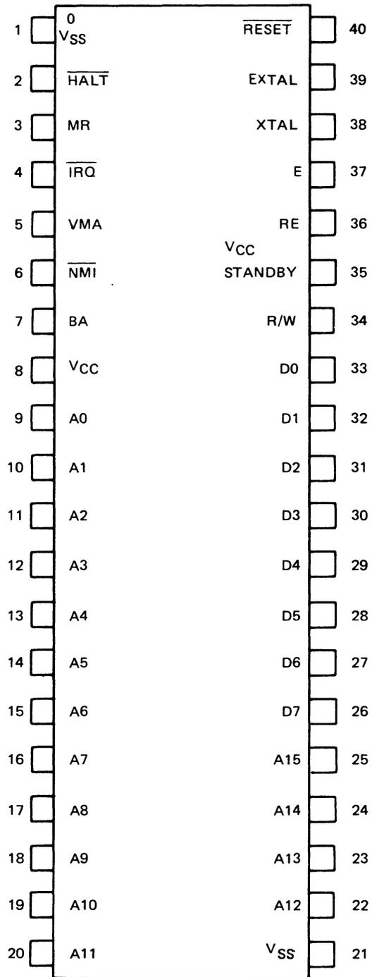
Figure 7-4. Microprocessor Pin Identification.
