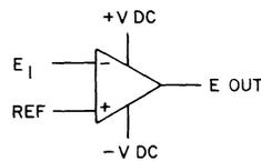
Figure 9-13.10. Voltage Comparator.
