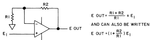
Figure 9-13.4. Noninverting Amplifier Gain Control.
