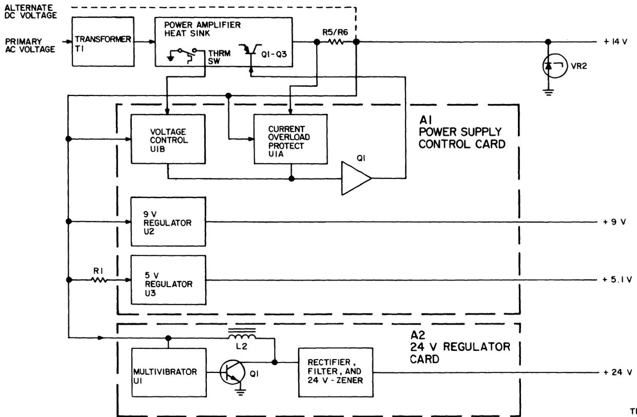
Figure 6-1. Power Supply Block Diagram.
