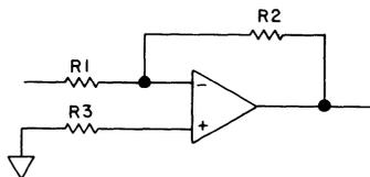
Figure 9-12.11. Differential Amplifier with Offset Correction.
