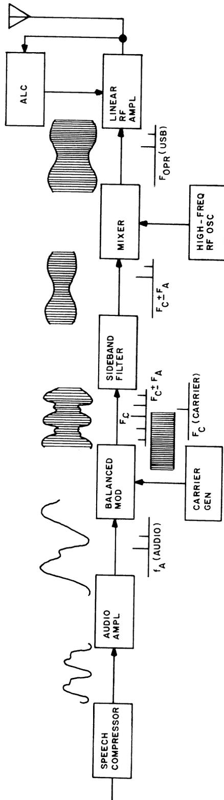
Figure 9-2.8. SSB Transmitter Simplified Block Diagram.
