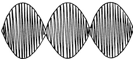
Figure 9-2.5. Single-Tone DSB or Two-Tone SSB Waveform.
