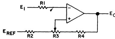
Figure 9-13.15. Voltage Comparator with Decreased Sensitivity.
