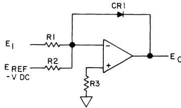
Figure 9-13.13. Voltage Comparator with Low Output Limiting.
