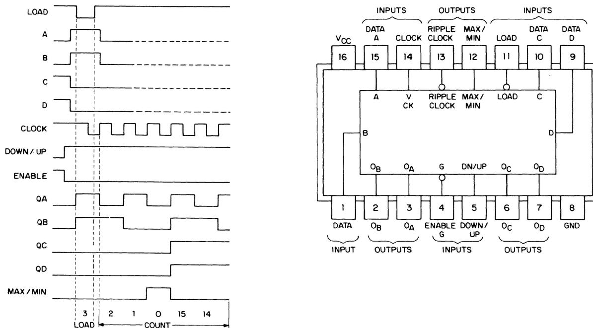
Figure 9-5.1. 74LS191 Count Sequence and Connection Diagram.
