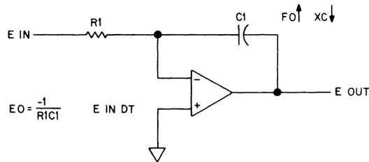
Figure 9-12.7. Integrator Circuit.
