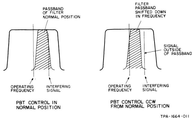
Figure 3-7. Passband Tuning to Eliminate Interfering Signal.
