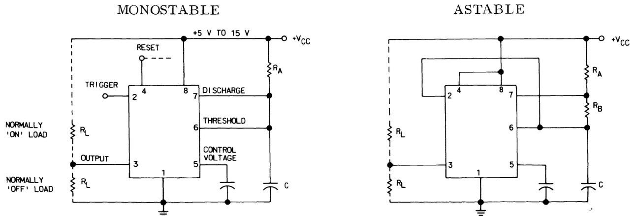
Figure 9-4.1. LM 555 Timer Diagram.
