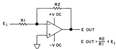
Figure 9-13.1. Inverting Amplifier.
