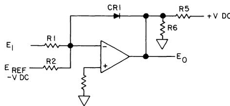
Figure 9-13.14. Voltage Comparator with Low and High Output Limiting.
