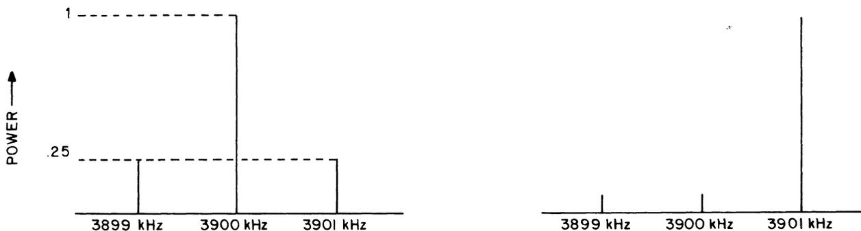
Figure 9-2.1. Comparison of AM and SSB Spectra.
