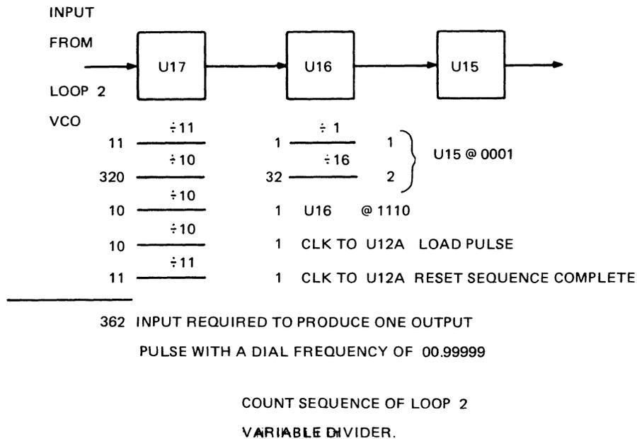
Figure 5-5. Count Sequence of the Loop 2 Variable Divider.
