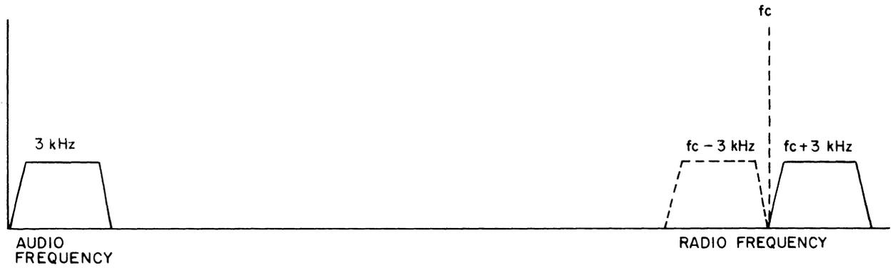
Figure 9-2.3. Location of SSB Signal in RF Spectrum.
