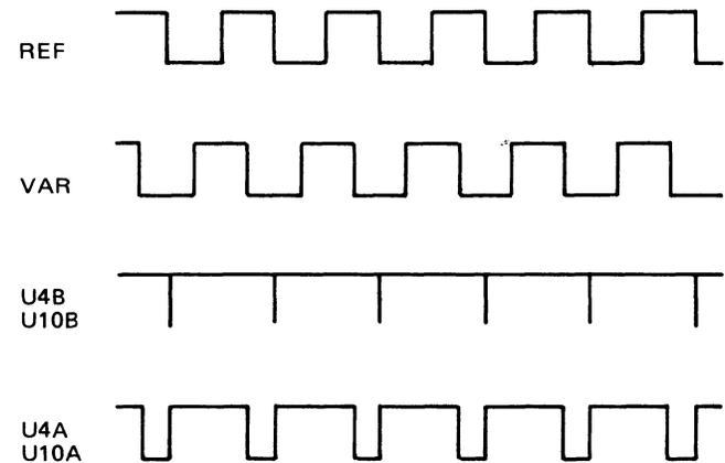
Figure 5-3. Loop 1 and 2 Frequency - Phase Detector Waveforms.
