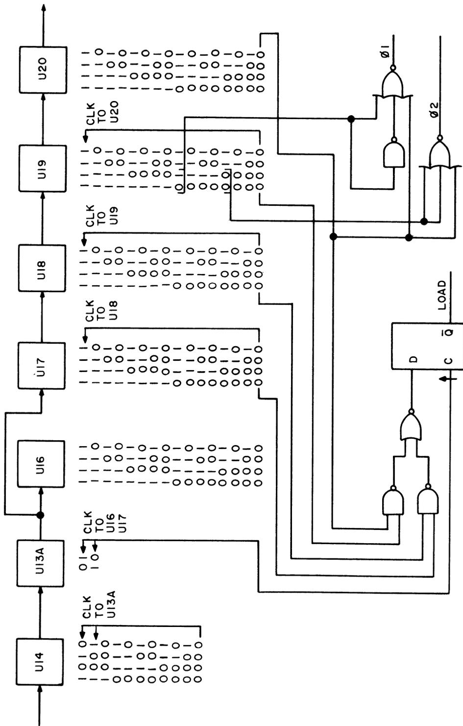
Figure 5-9. Internal Count Sequence and Output of the Variable Reference Loop Variable Divider.
