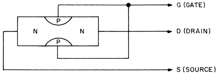
Figure 9-14.1. Cross Section View of an N-Channel Junction FET.
