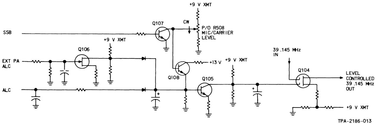
Figure 4-7. Exciter ALC Simplified Diagram.
