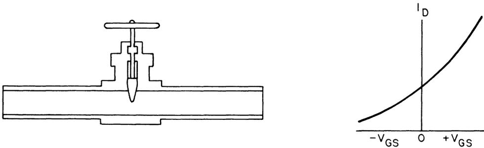
Figure 9-14.9. Depletion-Enhancement Characteristics.
