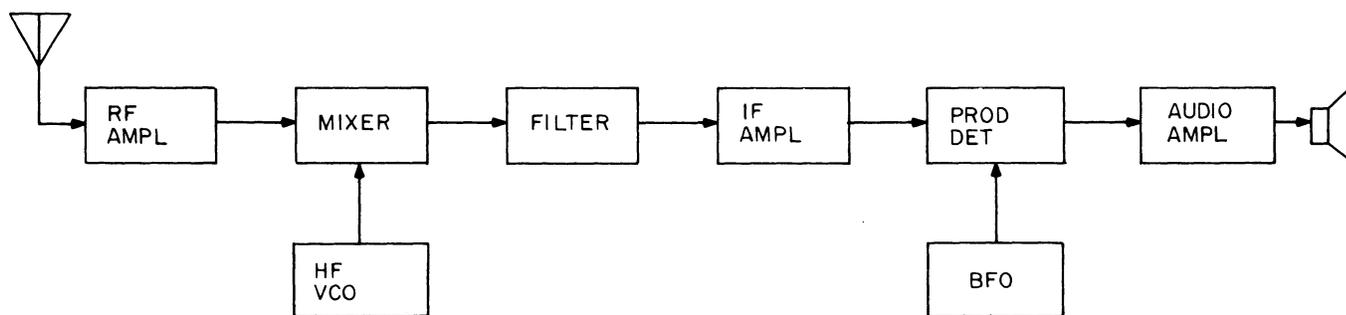
Figure 9-2.2. SSB Receiver Simplified Block Diagram.
