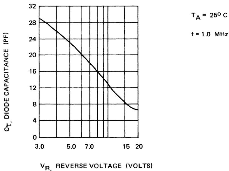
Figure 9-10.1. Voltage Variable Capacitor Reverse Voltage vs Capacitance Chart.
