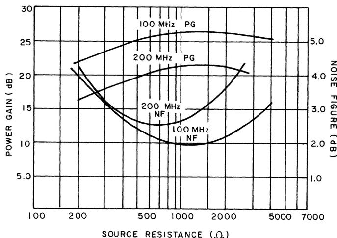
Figure 9-15.2. Dual-Gate Power Gain -- Source Resistance.
