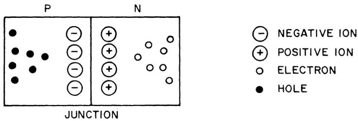
Figure 9-14.6. Formation of Potential Barrier at P-N Junction.
