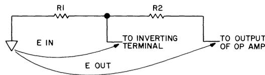
Figure 9-12.6. Resistive Divider Representing Noninverting Amplifier.
