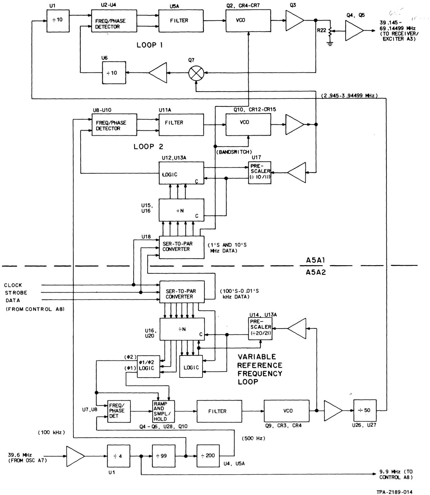
Figure 5-2. Synthesizer Block Diagram.
