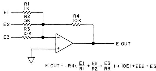
Figure 9-12.9. Scaling Adder.
