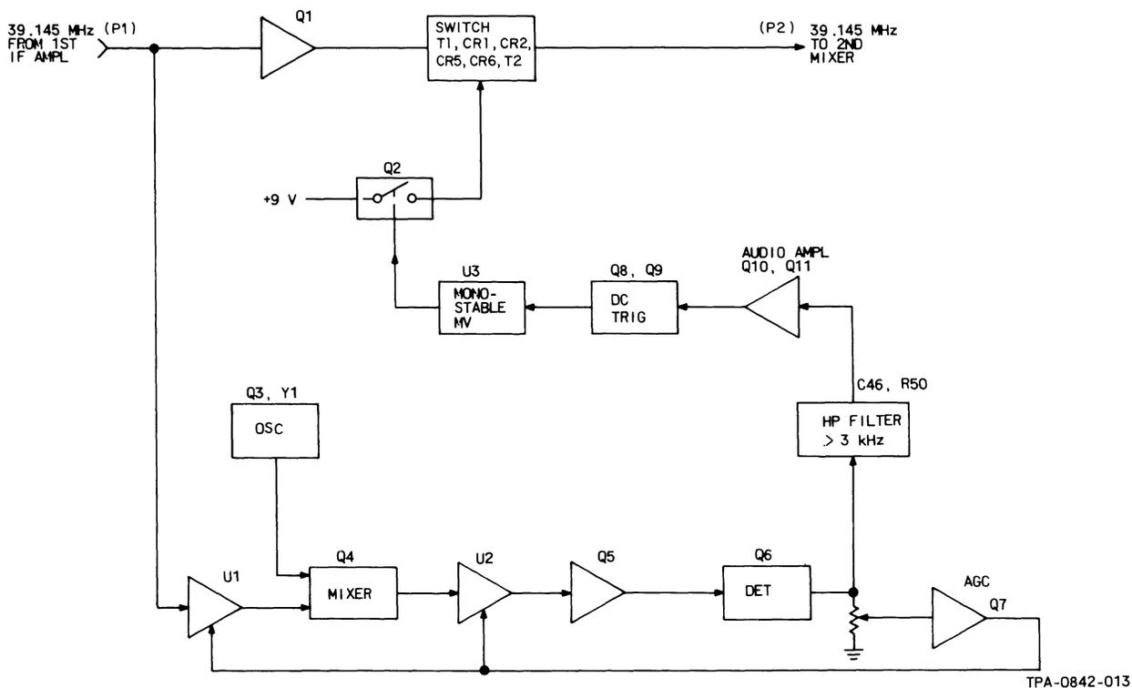
Figure 3-4. Noise Blanker Block Diagram.
