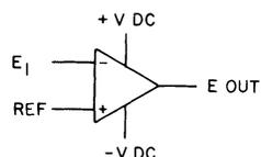
Figure 9-13.11. Voltage Comparator.
