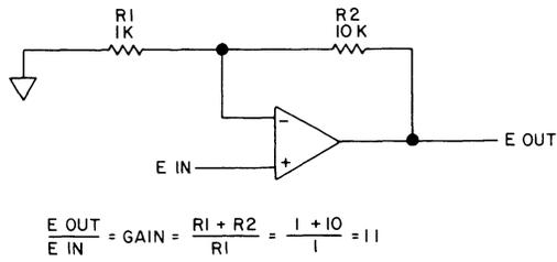
Figure 9-12.3. Noninverting Amplifier.
