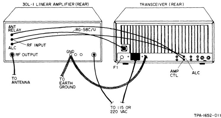
Figure 1-4. Interconnection for Transceiver and Linear Amplifier.
