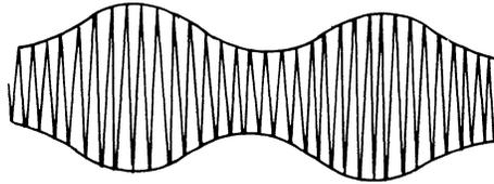
Figure 9-2.7. Single-Tone SSB Waveform with Pilot Carrier.
