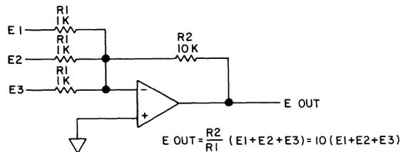
Figure 9-12.8. Voltage Adder.
