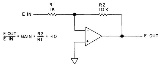
Figure 9-12.1. Inverting Amplifier.
