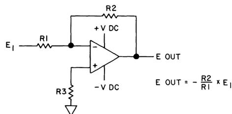
Figure 9-13.2. Inverting Amplifier with Added Temperature Stability.
